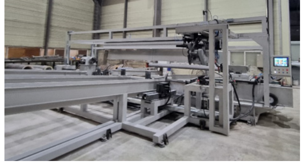
(a) Transfer automation device without pipe.
