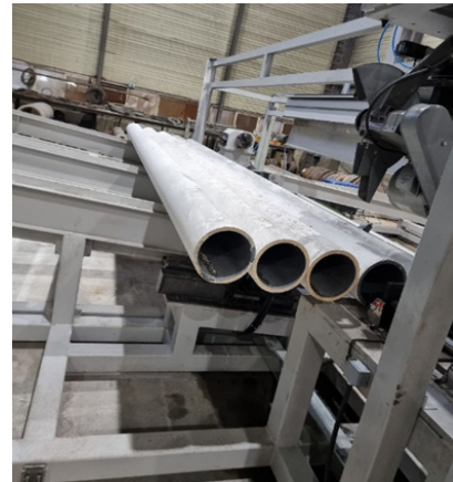
(b) Transfer automation device with pipe.
