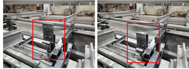
(a) Stopper 1 and its up and down movement without pipe.
